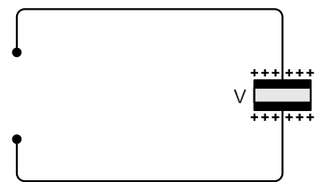
Fig. 5.15. Battery is removed across the parallel plate capacitor
